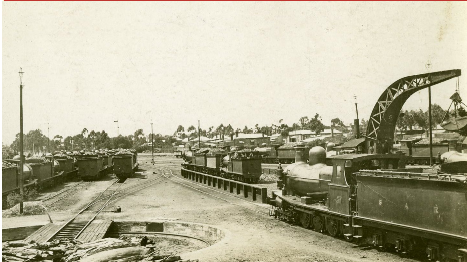
SAR Y class and T class steam locomotives at Peterborough loco depot, with portable coal, grab crane loading coal into tender of T class steam locomotive c1900
